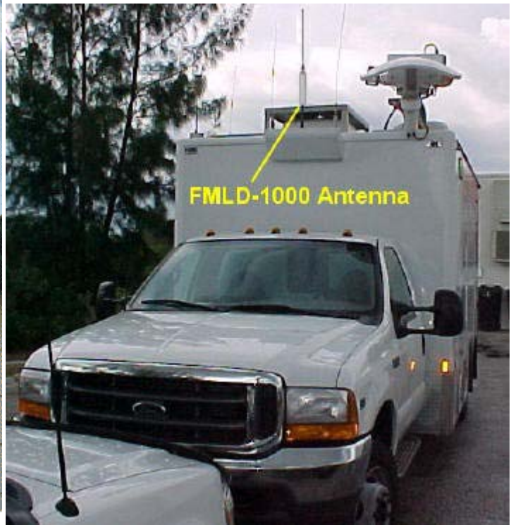
FMLD-1000 antenna mounted on TV Live Van
