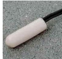
The heavy-duty probe has a 75-foot, PVC-jacketed and shielded cable with the sensor housed in a stainless steel cylinder (0.375" diameter, 1.50" length). It is designed to withstand the harsher outdoor environments.
