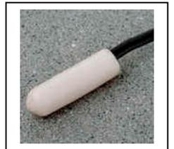
The **heavy-duty** probe has a 75-foot PVC-jacketed and shielded cable, with the sensor housed in a stainless steel cylinder (0.375" diameter, 1.50" length). It is well suited to withstand the elements of outdoor environments.
